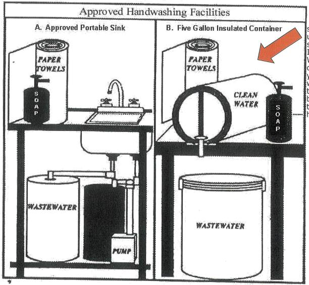
We suggest using this set up - an Insulated Water container for your hot water, paper towels, a bucket under the table and hand soap.
